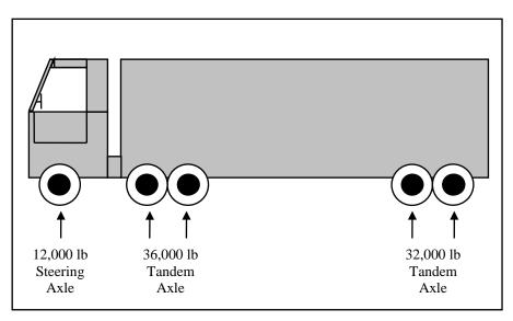
Figure 16. Semitrailer configuration 3-S2: the 18-wheeler.
