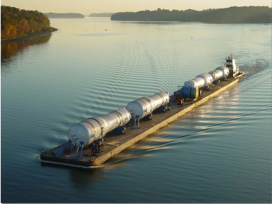
Figure 1: Steam Generators Moving to TVA's Watts Bar Nuclear Plant
